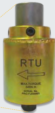
Modification of RTU for Track Bolt Tightening
